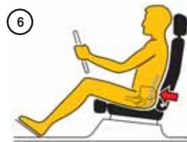
6 The RECARO Airmatic lumbar system is correctly adjusted when your lower spine is supported in its natural position.
