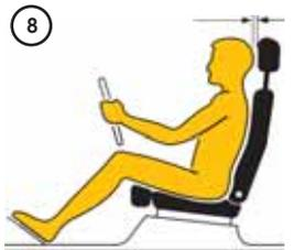
8 The top of the head rest should be set to exactly the same height as the top of your head. Tilt: the distance to the back of your head should be approx. 2 cm.
