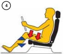
4 Adjust the seat cushion tilt so that the pedals can be depressed easily. Your thighs should rest lightly upon the seat cushion, without undue pressure. Check the seat back angle before moving off.
