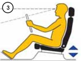
3 Set the seat height as high as possible. This ensures a clear view of the instruments and good all round vision.
